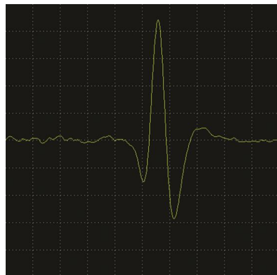
EC signal of the crack
